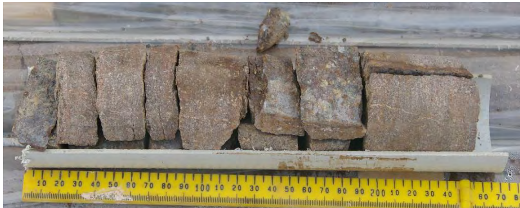
PHOTOGRAPH G7.13 Recovered core of slightly weathered, fractured basalt, Province 2, Muckaty Station
