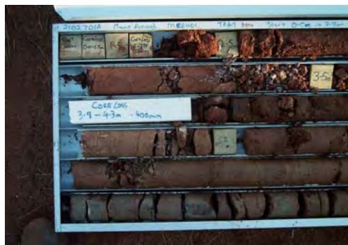
PHOTOGRAPH G7.1 Typical soil profile of calcareous sandy gravel overlying weathered sandstone
