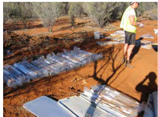
PHOTOGRAPH G4.4 Recovered rock core retained on PVC splits, wrapped in PVC tubing and stored in metal core boxes
