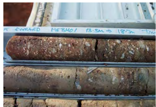
PHOTOGRAPH G7.2 Occasional Conglomerate beds encountered within the rock profile at Mount Everard
