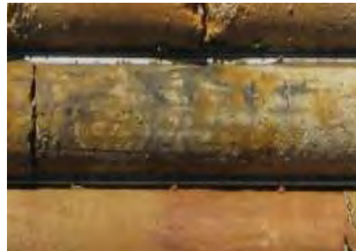
PHOTOGRAPH G7.3 Black veining (carbonaceous) encountered within the weathered Sandstone and occurred throughout the profile at Harts Range, beginning at approximately 25.5 m depth
