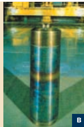
INNER CANISTERS: Height: 1.34m Diameter: 43cm
