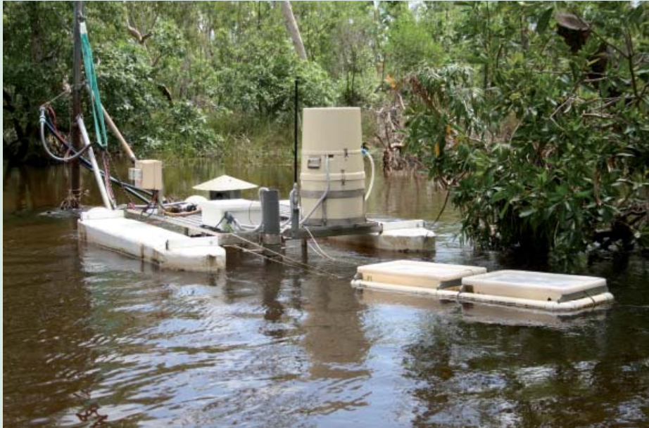
The SSD's continuous monitoring pontoon in Magela Creek downstream of the mine. The pontoon is equipped with two multiparameter (pH, electrical conductivity, turbidity) datasondes and an event-triggered autosampler. Source: Supervising Scientist Division, Department of the Environment, Water, Heritage and the Arts.
