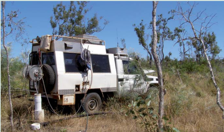
'The Lab Truck'—a purpose-built 4WD mounted environmental water quality sampling unit. Source: Northern Territory Government.
