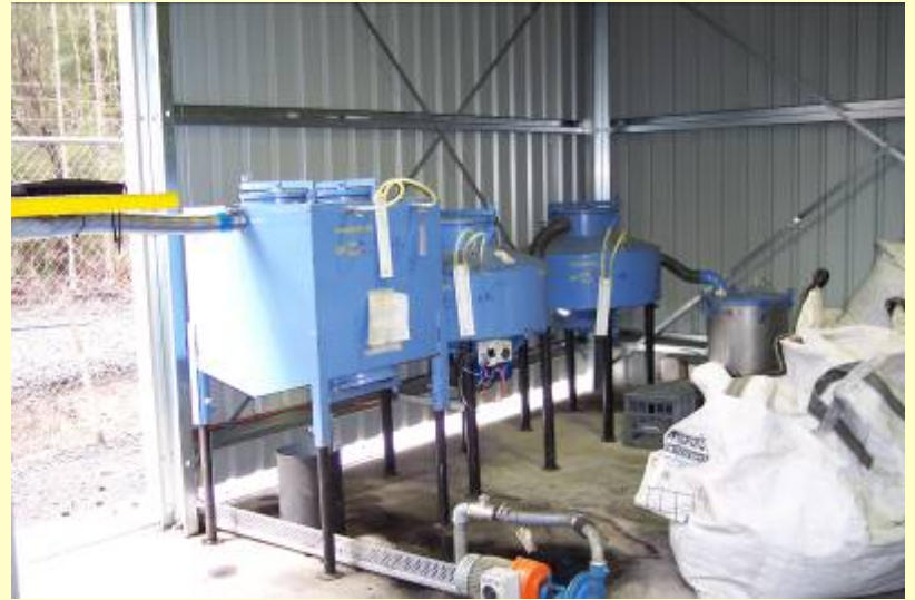
Ankur Gasifier dual firing a diesel genset - Huon Valley, Tasmania.
