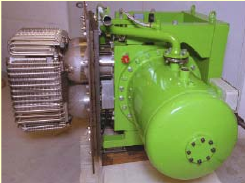
70 kW e Stirling engine - electric efficiency of ~12%. BIOS BIOENERGIESYSTEME GmbH, Austria
