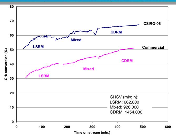
CSIRO solar reforming catalysts have significantly higher activity operating at 800°C compared to commercial reforming catalyst
