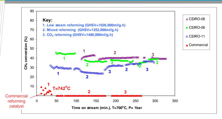
CSIRO solar reforming catalysts show excellent activity and stability for three reforming modes operating at 700°C as compared to commercial reforming catalyst operating at 742°C
