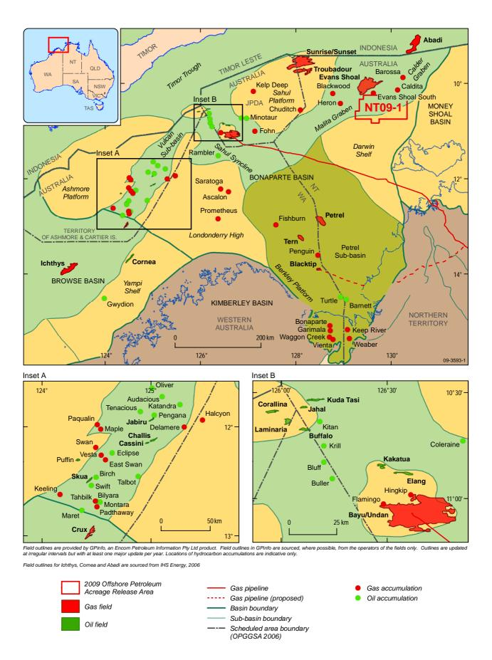
Figure 1. Structural elements map of the Bonaparte Basin showing location of the 2009 Release Areas and petroleum accumulations.
