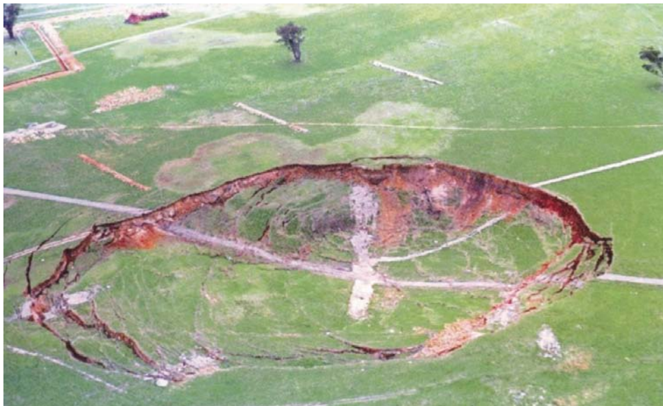
Figure 4.1 - An example of sustainability impacts of a mining operation - breakthrough of the Ridgeway sublevel cave - Orange, NSW, Australia
