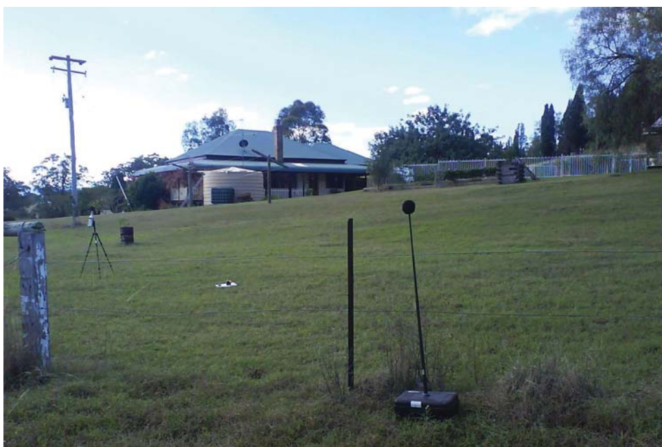
Figure 2.2 - Example of environmental noise logger in operation.
