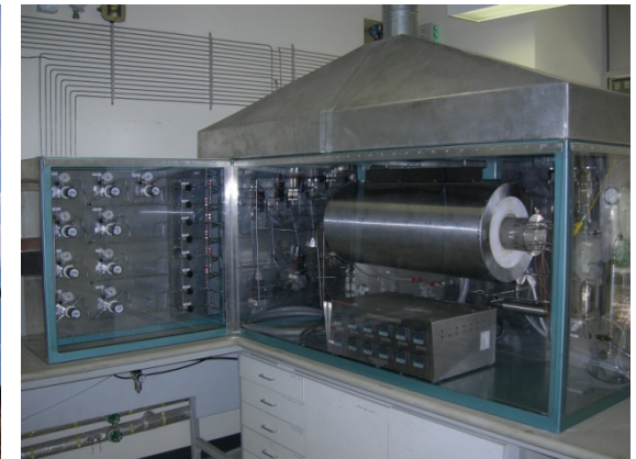
Membrane testing facility
