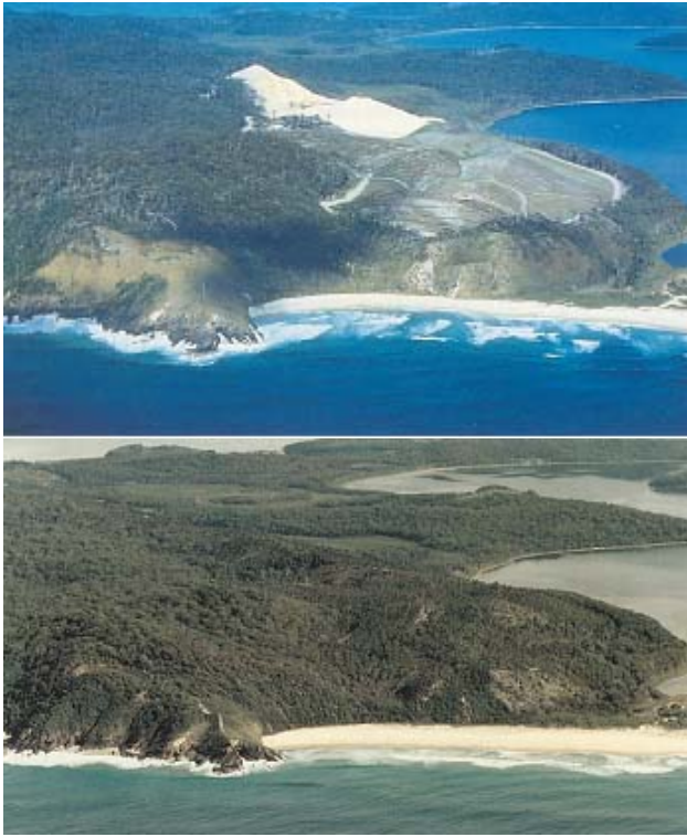
An area disturbed by mineral sand mining from 1974 to 1983 in the New South Wales coastal zone at Bridge Hill Ridge (above, taken in 1976), was rehabilitated and restored to a 120 metre high forested dune (below, taken in 1991). Photos: Yarwood & Associates
