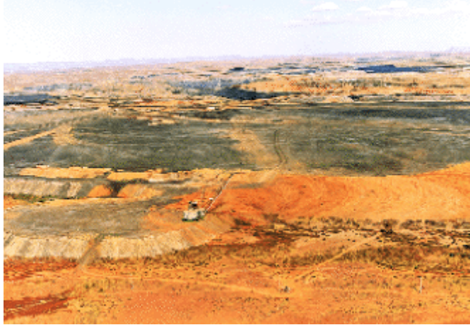
Photo: Optima Energy Page dragline adjusting dump slopes and cover with topsoil.
