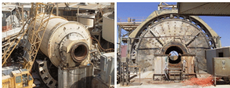
Ball mill number 2 removal
