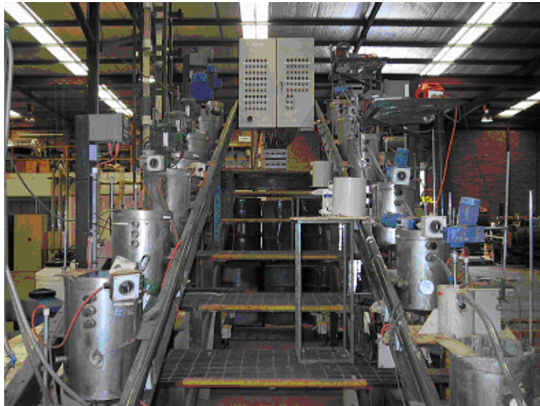
Typical pilot-scale cyanide detoxification set-up (photo: SGS Lakefield Orestest)
