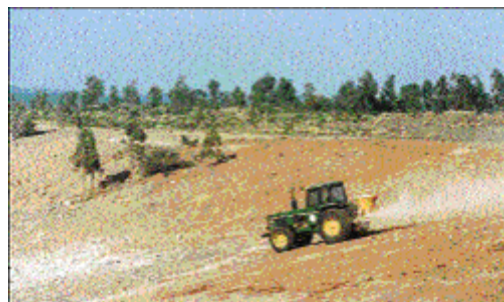
Figure 4: Red Dome Gold Mine, far North Queensland. Fertilising a recontoured waste rock dump prior to planting. (photo: Niugini Mining (Australasia) Pty Limited)
