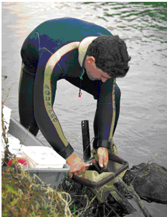
Biological Monitoring in the Ohinemuri River: artificial substrates are deployed for several weeks and then retrieved. The substrates consist of Perspex plates bolted together and then bolted on to a steel post in the river. A net is placed around the artificial substrate before it is removed from the post. In the photo you can see the waratah and the net. (Photo: Waihi Gold Mining Company Limited)
