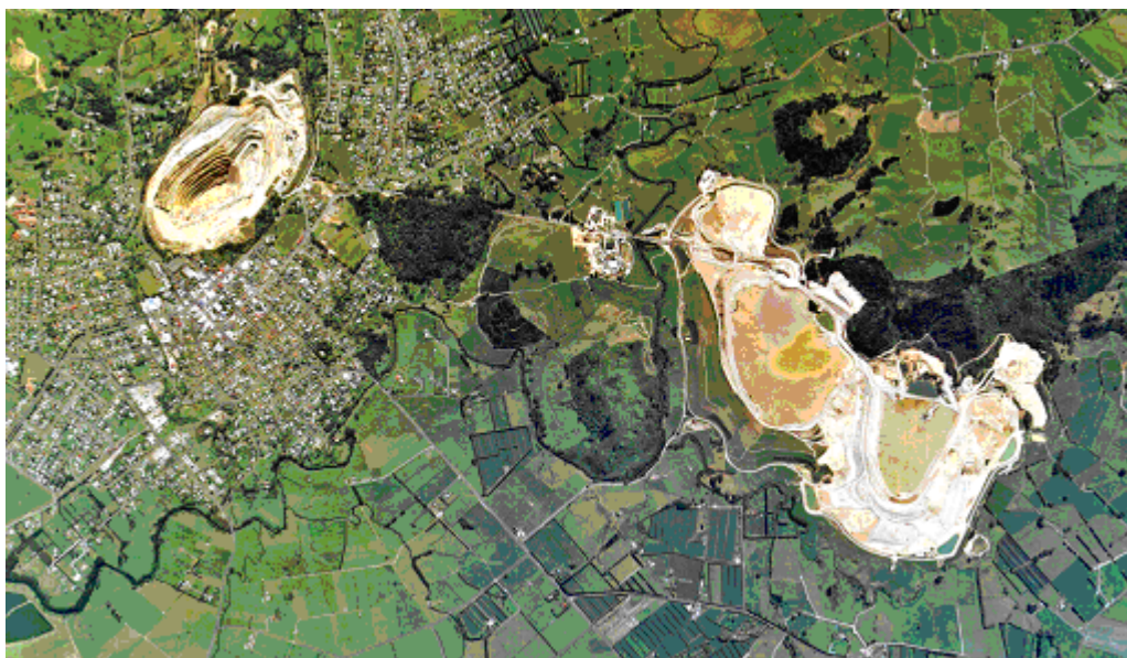
The Martha pit (top left) is surrounded by the town of Waihi. A conveyor transports ore to the processing plant (centre), and waste to the tailings storage facilities (centre right). The Ohinemuri River flows between the plant and the TSFs (photo: Waihi Gold Company Ltd).
