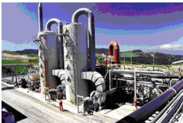
CYANISORB® (AVR) processor at Golden Cross Mine (photo: Coeur Gold New Zealand Ltd and Viking Mining Ltd).
