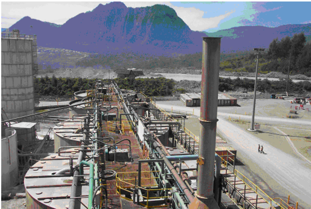
View across 4 of the 5 waste treatment circuit tanks at Porgera, where cyanide is precipitated as insoluble metal complexes. Looking towards discharge end; lime tank on left; Mt Paiam in distance (photo: Placer Dome Asia Pacific).
