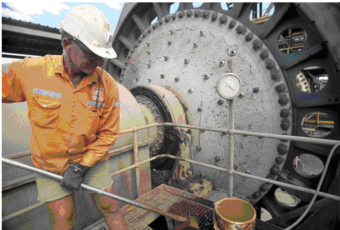
Discharge from the mill is regularly sampled to determine paste density
