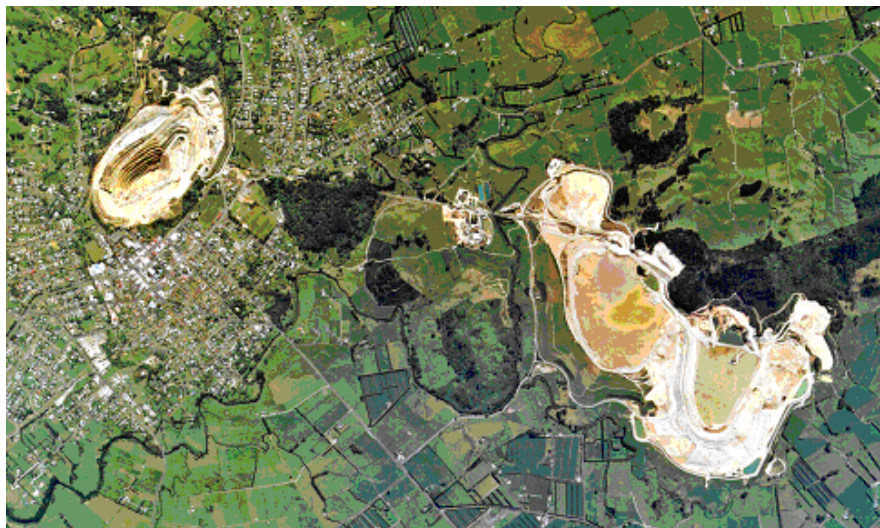
The Martha pit (top left) is surrounded by the town of Waihi. A conveyor transports ore to the processing plant (centre), and waste to the tailings storage facilities (centre right). The Ohinemuri River flows between the plant and the TSFs (photo: Waihi Gold Company Ltd).
