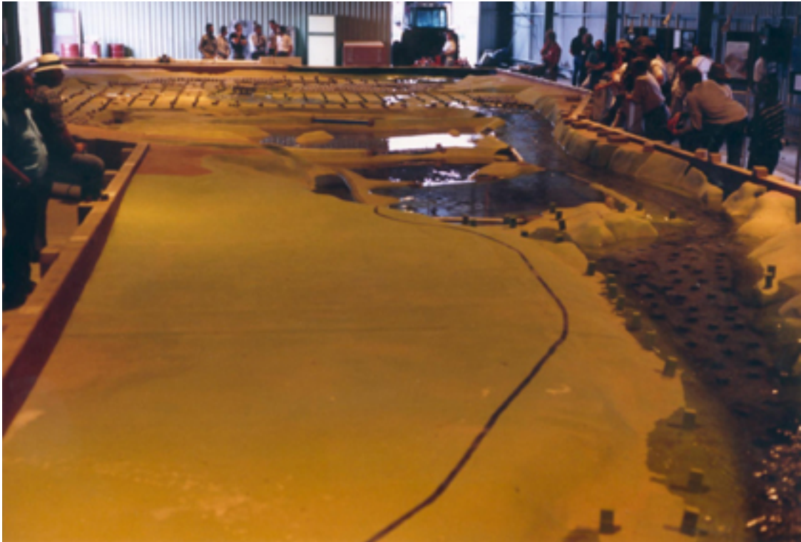
Physical Scale Surface Water Model for Penrith Lakes Development (October 1990)
