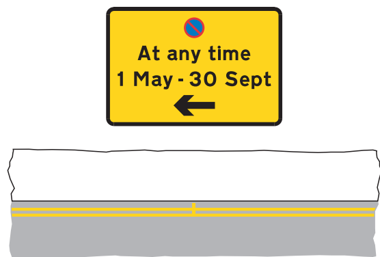
Figure 6-4 Change from seasonal no waiting at any time to all year round no waiting at any time
