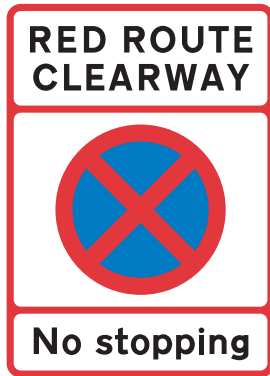
Figure 10-12 No stopping on red route clearway
