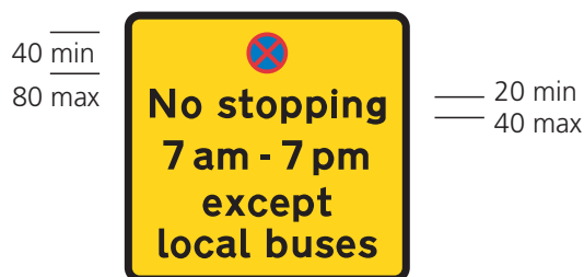
974 Place where only buses may stop during the period indicated, for the purpose of picking up and setting down passengers
