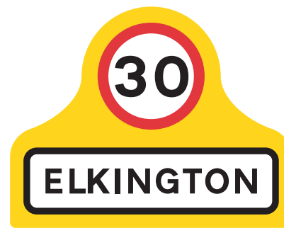
Figure 14-22 Example of a speed limit sign co-located with a boundary sign
