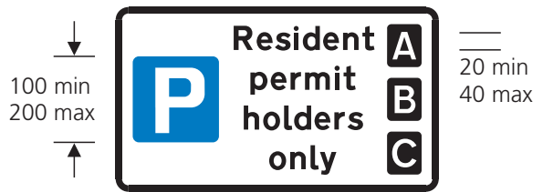
660.3 Parking place for resident permit holders
