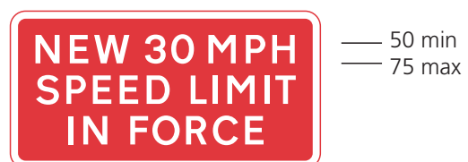
7032 Temporary sign indicating the start of a newly imposed 30mph speed limit which is contiguous to an existing 30mph speed limit
