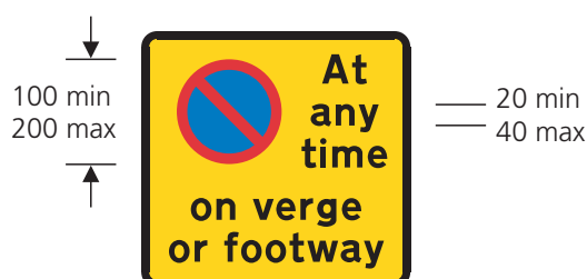
637.1 Continuous prohibition of waiting on verge or footway
