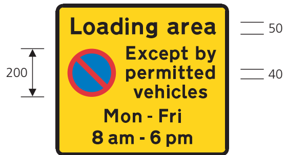
640.3 Entrance to a designated off-highway loading area in which waiting restrictions apply
