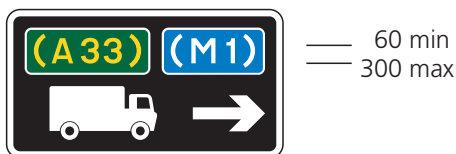
2805 Advance direction sign indicating a route advised for goods vehicles
