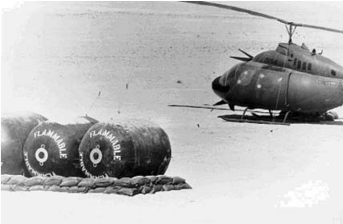
During a Gulf War deception operation a simulated OH-58C Kiowa helicopter with simulated fuel blivets was used to portray a forward arming and refueling point.
