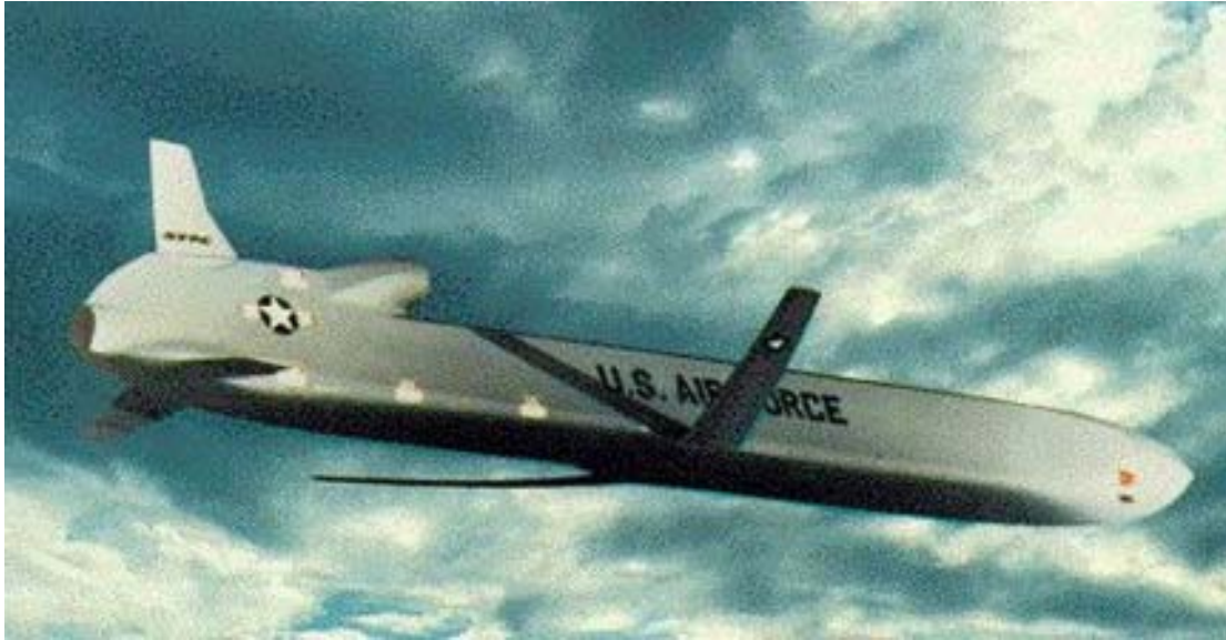
The conventional air-launched cruise missile is a near-precision Global Positioning System aided stand-off missile that can operate in varying threat environments and is ideally suited for high value targets and as a first-strike enabler for follow-on operations.
