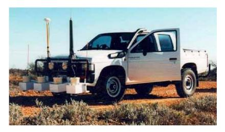
Figure 3. Nissan vehicle-mounted particle detection system
