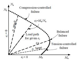
Fig. (1). Different failure modes for column under combined bending and axial load.
