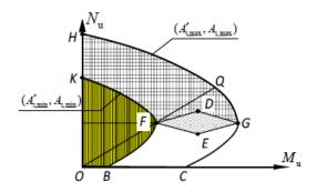
Fig. (4). Specified domains in interaction diagram.
