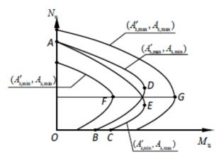
Fig. (3). Interaction diagram of column with maximum or minimum reinforcement ratio.
