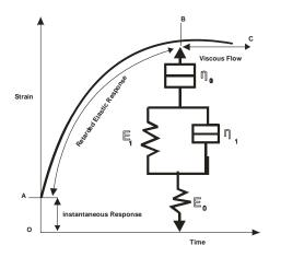
Fig.1: Mechanical Analogy of Four Element Burger's Model for a Typical Biological Material
