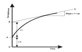
Fig.4: Graphical illustration for calculation of creep parameters
