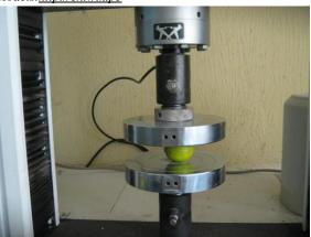
Fig. 1: Lime undergoing quasi-static compression
