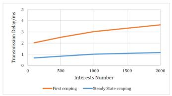
Figure 5: Measured transmission delay for ICN-SDN network
