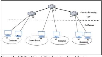
Figure 4: ICN-Traditional-Simple network architecture VI. Evaluation and Results
