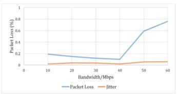
Figure 10: Packet Loss and Jitter Measured for ICN-Traditional Network
