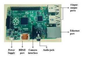
Fig. 5 Raspberry pi 2 Board
