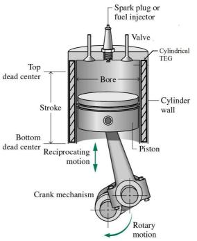
Fig.2 Engine Cross-section with Cylindrical TEG
