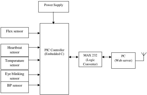
Fig. 3.1 Block diagram of the project
