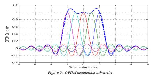
This method performs encoding digital data on multiple carrier frequencies.
