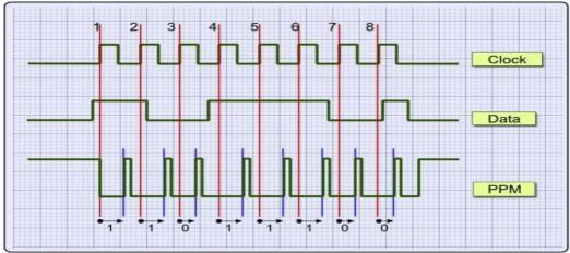
Figure 8: Shape of pulse position modulation
