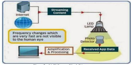
Figure2 : Li-Fi System Block Diagram
