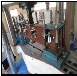
Fig.4 Lateral torsional buckling on NPI-125 (Hexagonal)
