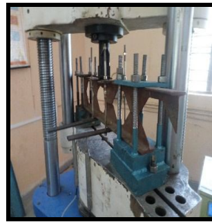
Fig.4 Lateral torsional buckling on NPI-125 (Hexagonal)
