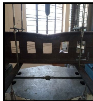
Fig.6 Lateral torsional buckling on NPI-125 (Square)
