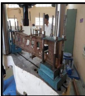
Fig.6 Lateral torsional buckling on NPI-125 (Square)
