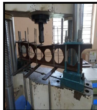
Fig.5 Lateral torsional buckling on NPI-125 (Circular)
