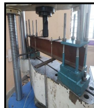
Fig.7 Lateral torsional buckling on NPI-125 (Plane)
