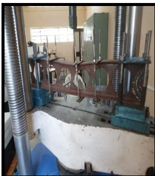
Fig.5 Lateral torsional buckling on NPI-125 (Circular)
