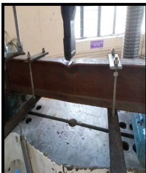
Fig.7 Lateral torsional buckling on NPI-125 (Plane)
