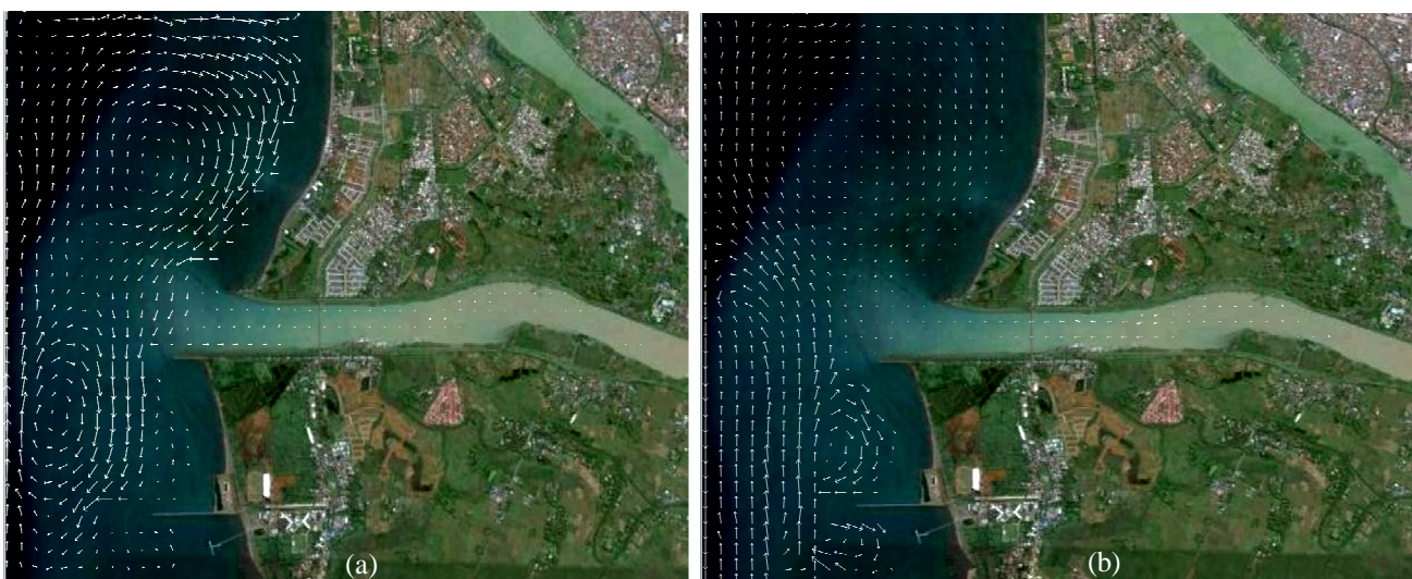
Fig. 1 Current pattern without the Jeneberang rubber dam overflow discharge, (a) Spring tide flow condition, (b) Low tide flow condition
