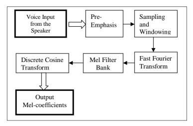
Fig 1 Block diagram for obtaining MFC coefficients
