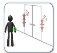
An example of the anti-wandering wristband based door alarm system
