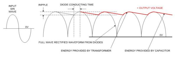
Fig. 3 Smoothing capacitor characteristics
