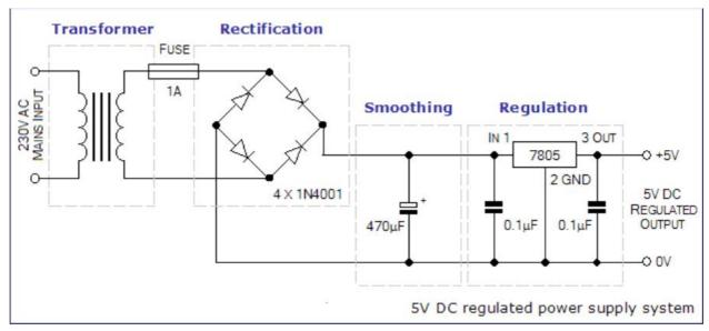
Fig. 2 Typical power supply section
