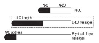
Fig. (2). Message structure of BACnet Ethernet communication protocol.
