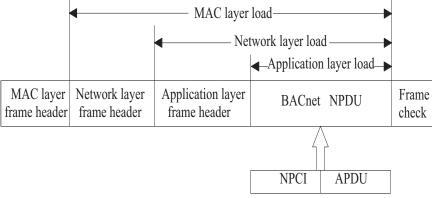
Fig. (4). BACnet protocol message encapsulation in ZigBee network.
