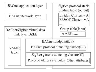
Fig. (3). BACnet/ZigBee interconnection mechanism based on BZLL.
