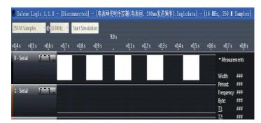
Fig. (8). Logic analyzer display YD2010 device response byte.
