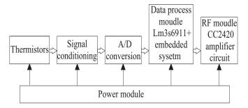
Fig. (5). BACnet/ZigBee node hardware schematic.
