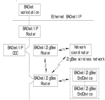
Fig. (1). BACnet/ZigBee communication network structure.
