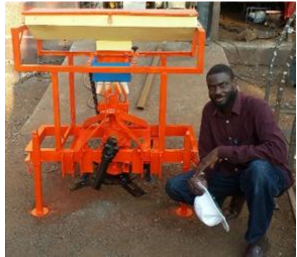
Fig (3) Ratoon Implement front view
