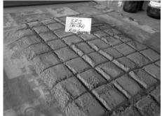
Figure 1. Composite sample of flotation tailings prepared for experimental testing
