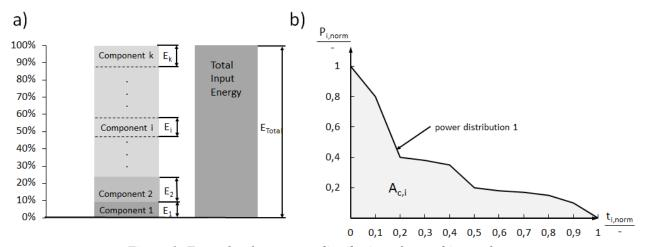
Figure 1: Example of an energy distribution of a machine tool.
