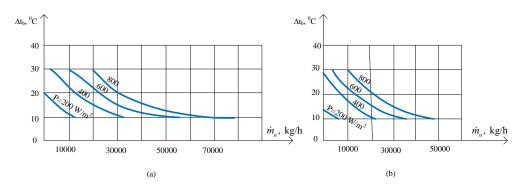
Fig. 6. Dependence of change  $\dot{m}_a$  from  $\Delta t_b$  for k=5,8 W/(m<sup>2</sup>K) and (a):  $(\tau \alpha)=0,73$  and (b):  $(\tau \alpha)=0,55$
