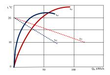
Fig. 1. Dependence  $Q_b$  from  $t_h$  and  $t_o$  for the glass with constructive certain features, with one glass (1) and double glass (2),  $k_1 = 5.8$  W/(m<sup>2</sup>K),  $k_2=3.6$  W/(m<sup>2</sup>K),  $t_b=20^{\circ}$ C,  $\dot{m}_a = 6.25$  m<sup>3</sup>/s, S<sub>m</sub>=1950 m<sup>2</sup>
