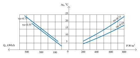
Fig. 5. Dependence of change  $Q_s$  from P and  $\Delta t_b$  for glass with k=5,8 W/(m<sup>2</sup>K),  $\dot{m}_a = 6,25 \text{ m}^3/\text{s}$  and  $t_o = 20^{\circ}C$ .
