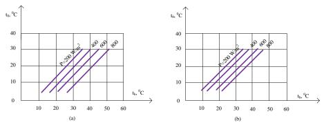
Fig. 4. Dependence of change  $t_{vs}$  from  $t_o$  and P for k=5,8 W/( $m^2K$ ); (a): ( $\tau\alpha$ )=0.73, and(b): ( $\tau\alpha$ )=0.55
