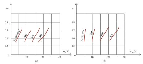
Fig. 3. Dependence of change  $\Delta t_a$  from P and  $(\tau \alpha)$  for (a) k=5,8 W/(m<sup>2</sup>K) and (b) k=3,6 W/(m<sup>2</sup>K), and glass with certain characteristics.
