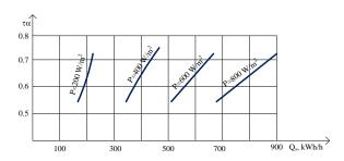
Fig. 2. Dependence of change  $Q_s$  from ( $\tau \alpha$ ) for different values of P, and for  $S_{bm}$ =1540 m<sup>2</sup>
