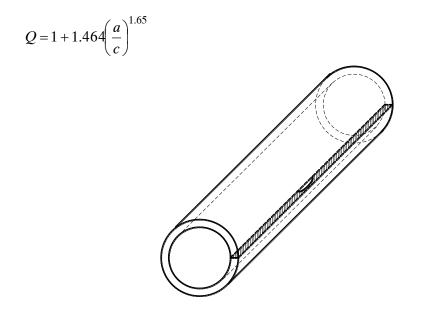
Figure 1. Pipe with longitudinal internal surface crack
