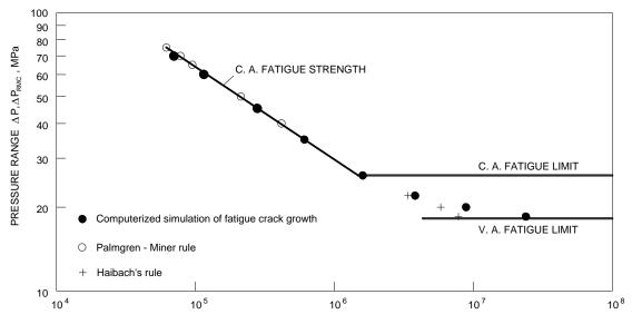
CYCLES TO FAILURE
