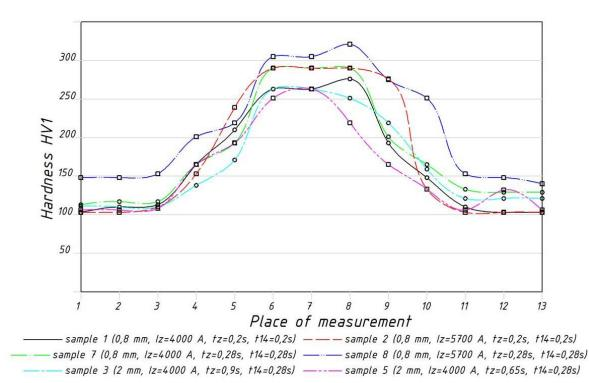
Figure 4. Hardness distribution in weld nugget and HAZ [6]
