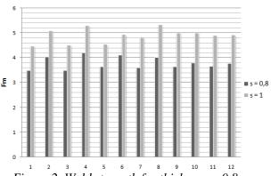
Figure 2. Weld strength for thicknesses 0,8mm and 1mm.
