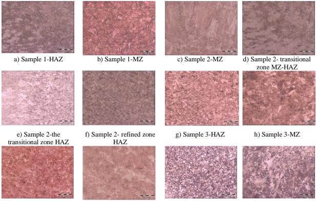
i) Sample 5-HAZ j) Sample 5-Melting zone k) Sample 7- HAZ l) Sample 7- MZ Figure 5. Microstructure of the weld nugget and heat affected zone[6] (Samples designated as in Figure 4)
