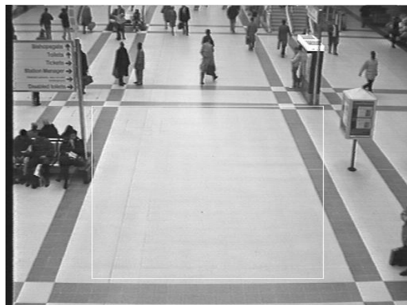
Fig. 3: A “background-only” image for the site in Fig. 3. This is used to isolate pedestrians from images by removing the surrounding background.
