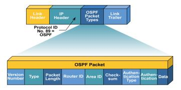
Figure 2.1: OSPF Message encapsulation. (Cisco Press "OSPF Message Encapsulation", 1999)
