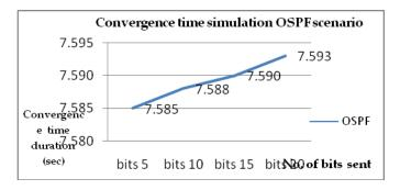
Figure5: Convergence time simulation graph for OSPF (above)
