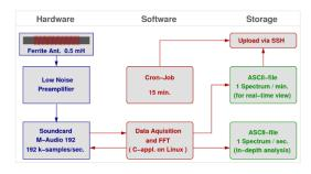
Fig 1: Block diagram of Kiel Longwave Monitor
