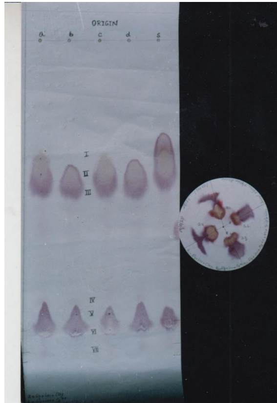
Fig B: Chromatogram showing the formation of peptides from reaction system of Glycine and Leucine heated upto 150 hrs.
