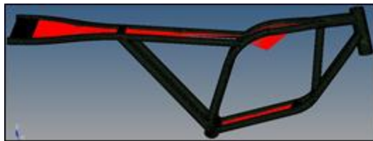
Fig. 5. Loads Applied On Chassis In Hypermesh
