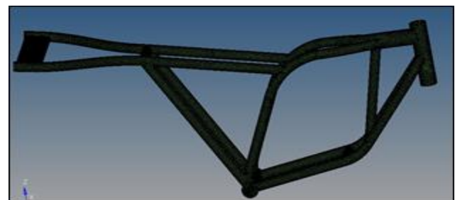
Fig. 4. Meshed Model of Bike Chassis The properties of mild steel are listed below:
