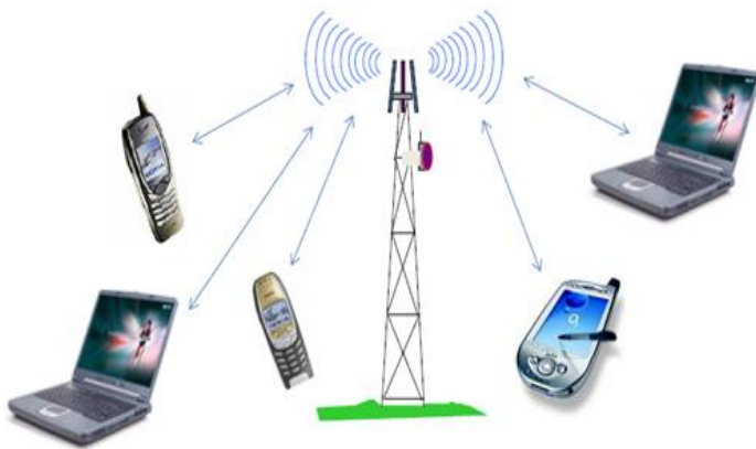
Fig.1. Infrastructure Network Model
