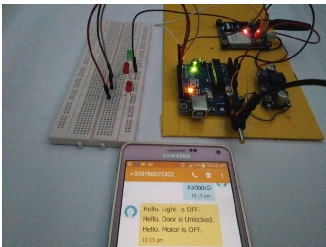
Figure: Experimental Result when three home appliances are turn off
