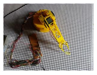
Figure 8; experimental testing the robot arm to reach at position 1
