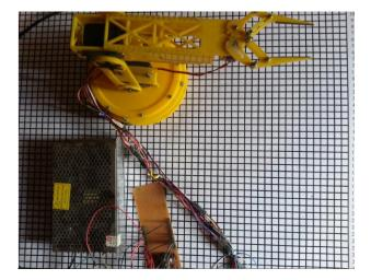
Figure 7; testing the robot arm at home position (all servo angles are 90° applied)
