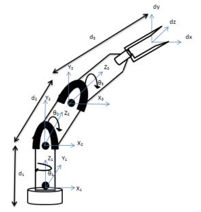
Figure 3; Link parameters of articulated robot manipulator
