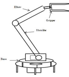
Figure 1: Structure of articulated robot arm design
