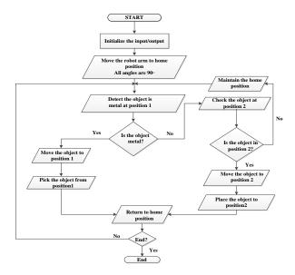
FIGURE 6; FLOW CHART OF PICK AND PLACE ARTICULATED ROBOT ARM
