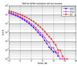
Figure4.BER performance with qpsk modulation in SC,MRC,EGC
