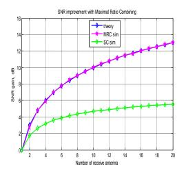
Figure 3. SNR improvement using MRC and SC
