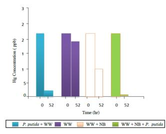
Figure 4: Mercury removal by P. putida in petroleum based industries wastewater
