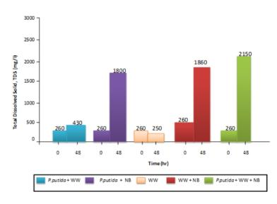
Figure 5: Effect of P. putida growth to total dissolved solid of petroleum based industries wastewater
