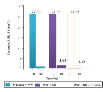
Figure 6: Effect of P. putida growth to suspended solid of petroleum based industries wastewater
