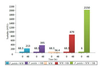
Figure 7: Effect of P. putida growth to turbidity of petroleum based industries wastewater
