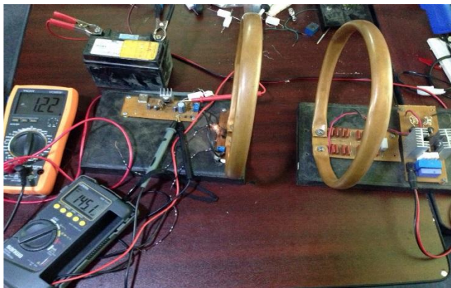
Fig. 17. DC Voltage and Ampere (between transmitter and receiver=4inches) P=VI=145.1m*1.22=0.18W (Loading 10Ω,5W)
