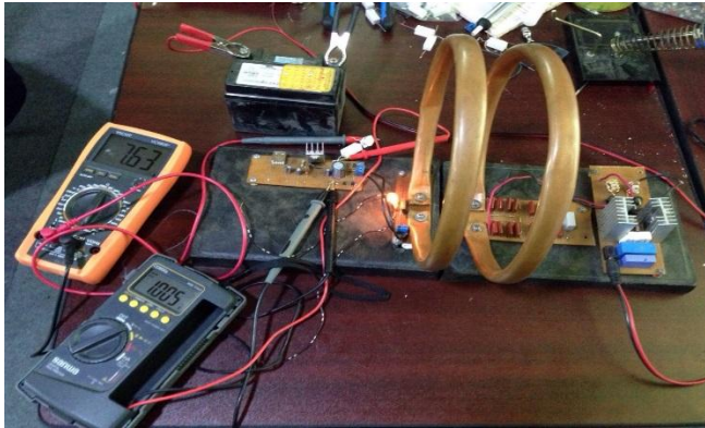
Fig. 16. DC Voltage and Ampere (between transmitter and receiver=1.3inches) P=VI=1.005*7.63=7.4W (Loading 10Ω,5W)
