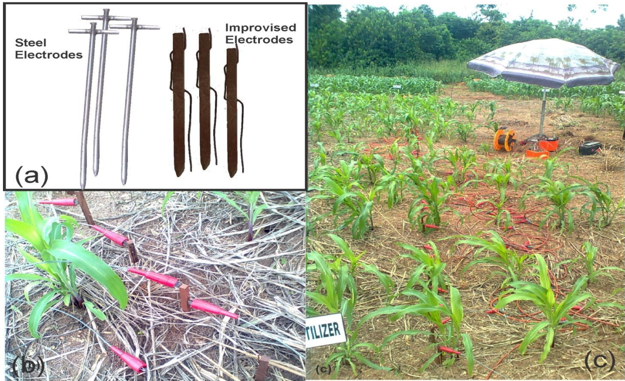
Fig. 3: (a) Electrodes (b) Cable-jumper- electrodes connection (c) Set-up of system for CVES measurements.
