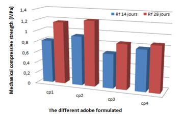
Fig.5. Mechanical compressive strength of adobe made
