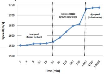
Fig.8. Changes in the speed of wave propagation as a function of moisture.
