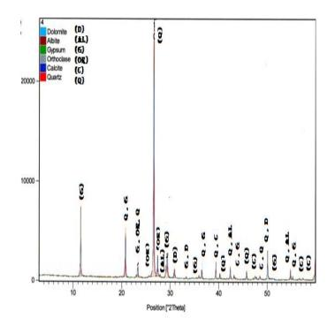
Fig .2. Mineralogical analysis of sand dune
