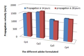
Fig.6. Histograms of time and speeds adobes made by the ultrasonic test.
