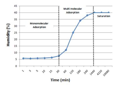
Fig. 7. Evolution of moisture as a function of time
