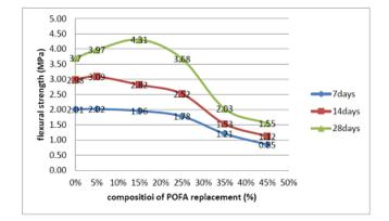
Figure 4: Average flexural strength verses curing days of concrete specimens
