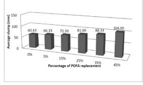
Figure 1: Results of Slump Test
