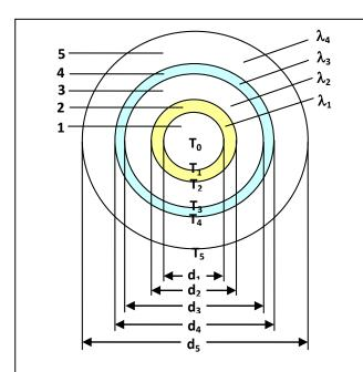
**Fig. 1.** Geometrical design of the cross-section of the laser tube of a new He-SrBr<sub>2</sub> laser: 1 – discharge, 2 – ceramic (Al<sub>2</sub>O<sub>3</sub>) tube, 3 – space filled with helium or other material, 4 –quartz tube and 5 – insulation. The diameters are as follows:  $d_1 = 30.5 \, \mathrm{mm}$ ,  $d_2 = 38.6 \, \mathrm{mm}$ ,  $d_3 = 71 \, \mathrm{mm}$ ,  $d_4 = 75 \, \mathrm{mm}$  and  $d_5$  - diameter of the insulation.
