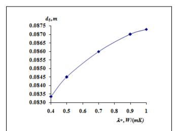
Fig. 3. Dependence between the insulation diameter  $d_5$  and the heat conductivity coefficient  $\lambda^*$  of the searched material between the ceramic and quartz tubes at fixed optimal gas temperature  $T_0$  in the centre of the tube.
